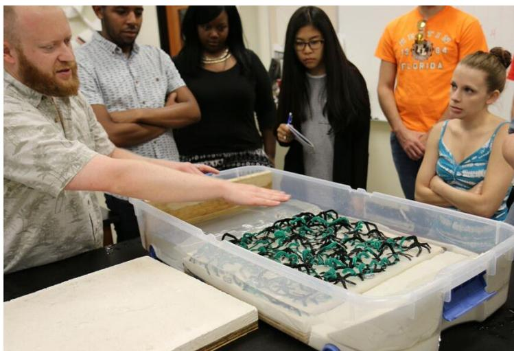
**Figure 5. Students add twisted pipe cleaners, which simulate the prop roots of mangroves, such as the red mangrove (*Rhizophora mangle*), to the simulated continental shelf to measure their impact on wave attenuation.**
