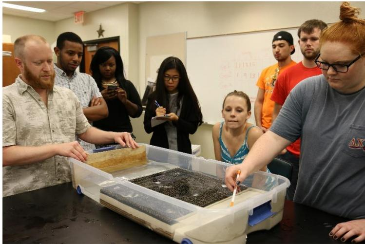
**Figure 4. Plastic doormat affixed to the top of the continental shelf to demonstrate wave energy attenuation of seagrass beds.**
